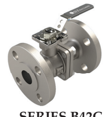
SERIES B42C ANSI Class 300 Fire-Safe API 607 Full Port Sizes from 1/2" to 8"
