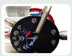
To switch to manual mode, the declutch bar is lifted and air is automatically released from the Actuator/Solenoid port and blocked from entering through the Pressurized Air Port. This simple and efficient release of air makes operation of the gear easier and safer.
