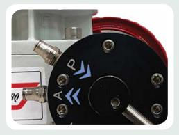
In auto mode, the actuator drives the valve using air entering through the Pressurized Air port and the Actuator/ Solenoid port.
