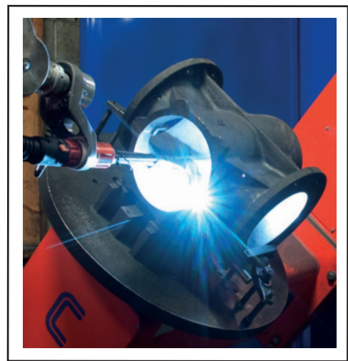
Figure 4. Robotic welding of nickel seat
