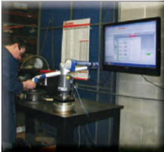
*Coordinate Measuring Machine provide 3D data*
