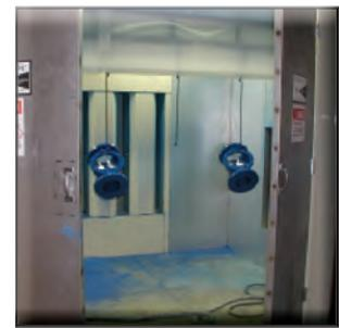
*Automated Electrostatic Fusion Bonded Epoxy Process*
