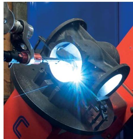
Figure 3. Robotic welding of nickel seat
